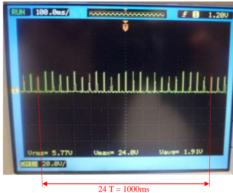
Figure 33: Oscilloscope screenshot: determination of the frequency: 1 peak corresponds to 1 contact
