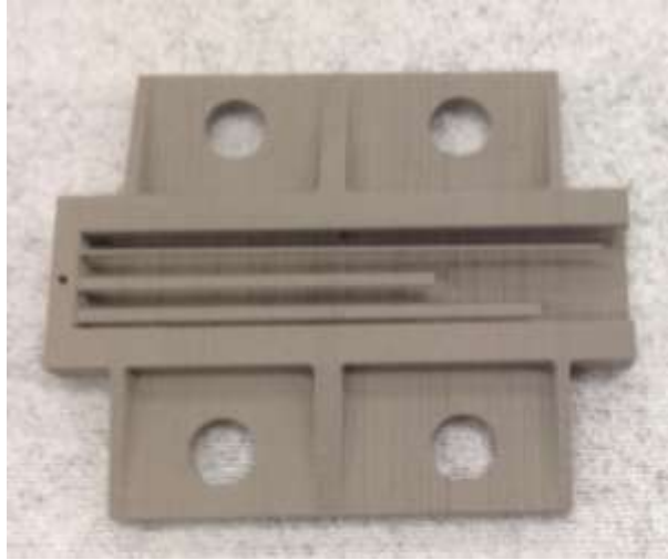
Figure 38: Metal vibration sensor after the cleaning phase
