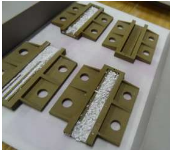
Figure 39: Metal vibration sensor: sintering preparation
